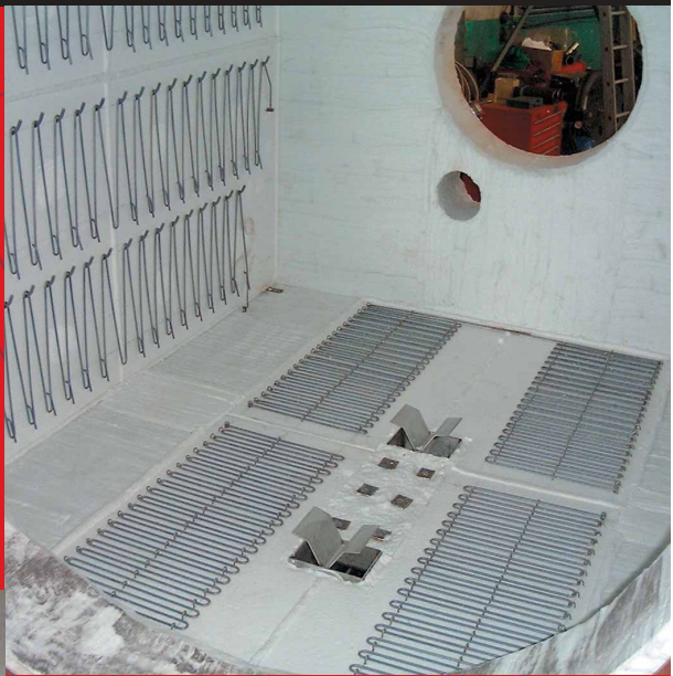
Electrical heating system of a chamber furnace. Heating elements in side and bottom mounted on vacuum preformed insulating parts.
