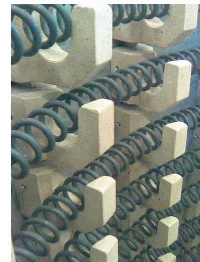
Heating cylinder of an air circulation furnace. Heating spirals mounted on appropriate perches.
